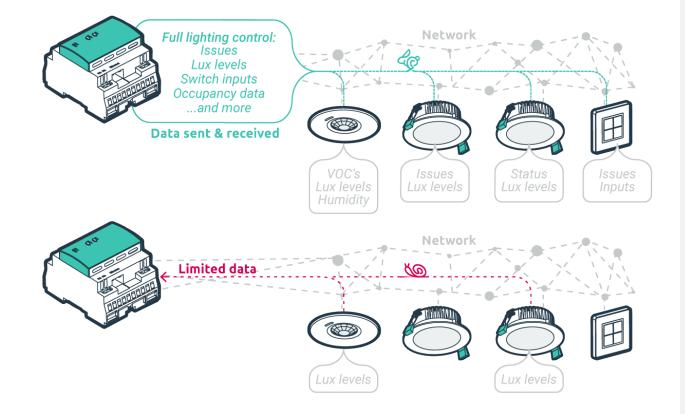
With IEC62386-104 over Thread<sup>®</sup>, we can provide a **fully functioning, no compromise lighting control system,** which allows full bandwidth control.
