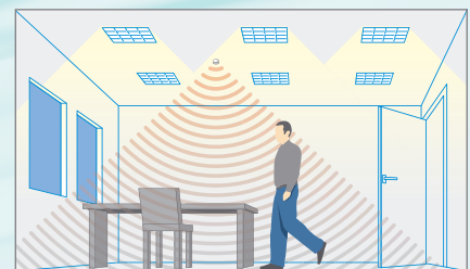
Presence detected, some daylight. Lights on and dimmed to maintain lux level.
