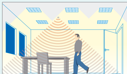
Presence detected, insufficient daylight, all lights on.
